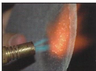
Actual disk of HeatShield Cerfractory heated with torch
